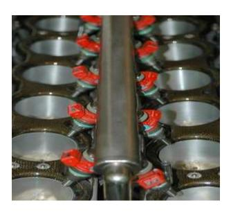
12. Fuel Injection system – Used in CI Engine
