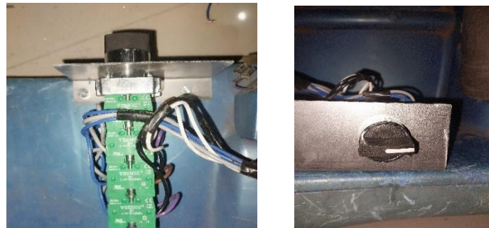
Figure 3: Change over switch used. First one is the side view and second view is the top view.
