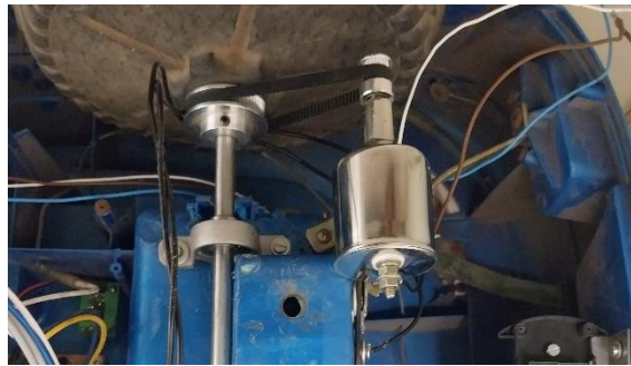
Figure 5: Dynamo's axle connected to the rotating shaft of the wheel using rotating gears.
