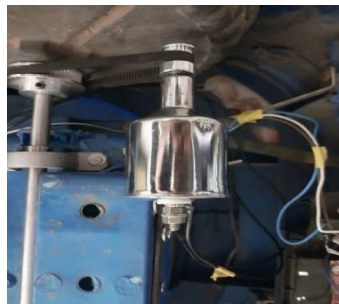
Figure 2: Dynamo used in the car to generate electricity.
