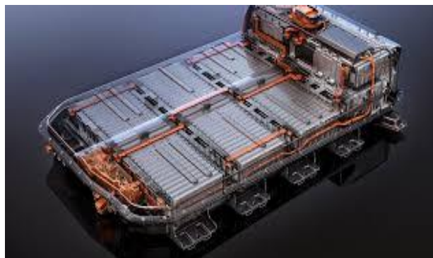
Figure 7: Two Layer battery mounted on the chasis of the EV.
